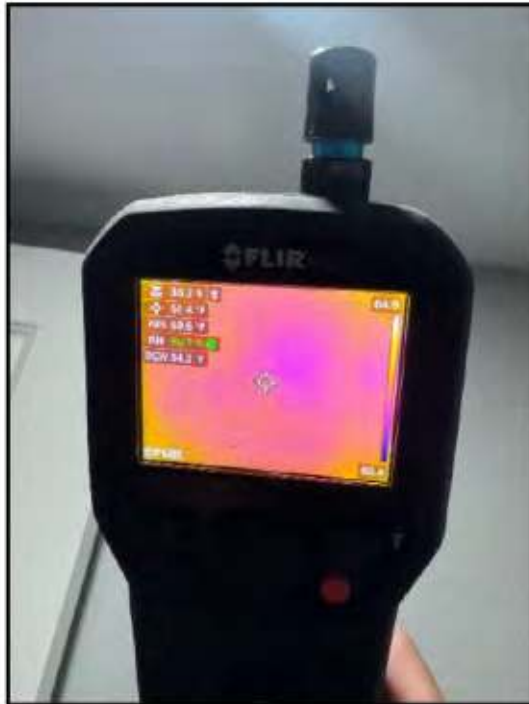
185. Active water leak detected
